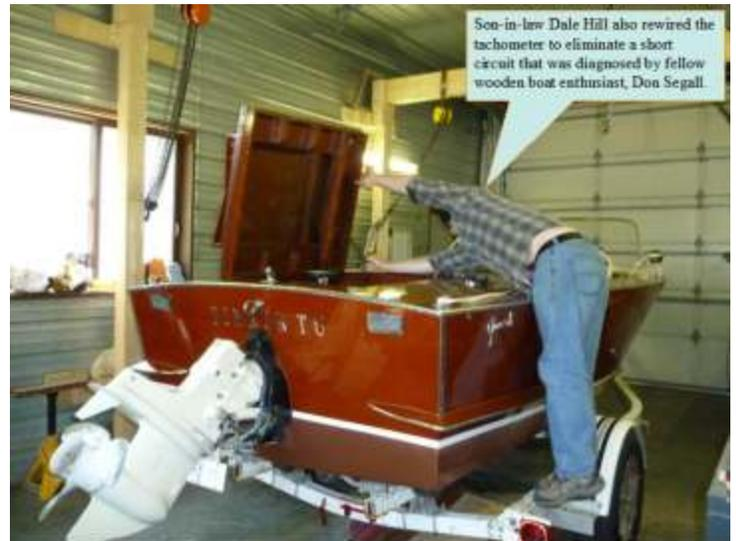
Tinker's restoration was now complete with all repairs done, 9 coats of varnish, 3 coats of copper paint on the bottom and 3 coats of Interlux boot-top paint on the waterline, a repainted Out/Drive, steering wheel and control box, new flooring and refinished interior.
